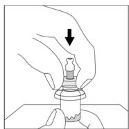
4. Swab the syringe connection point (blue circle) of the SmartSite<sup>®</sup> Access Device with preferred antiseptic prior to attaching the syringe to the SmartSite<sup>®</sup> Access Device.
